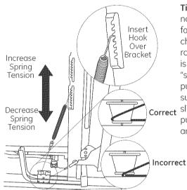
Tip: If door does not open easily or falls too quickly, check spring cable routing. The cable is held in place by "shoulders" on the pulley. Check to be sure cable has not slipped over the pulley shoulders and onto the axle.
